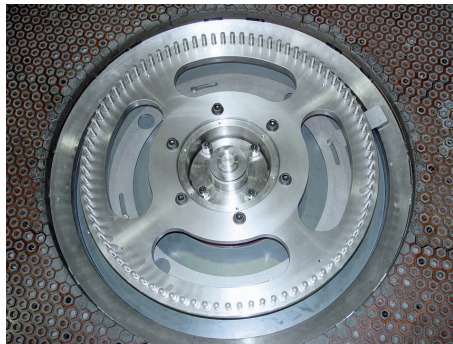
Measuring anvil, inner pin ring and segmented grinding wheel
