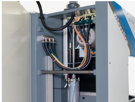
Swivel mounted switch cabinet for optimal machine accessibility
