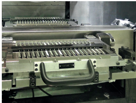
Index table with two clamping fixtures
