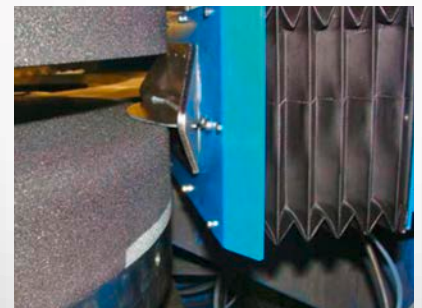
Sensor Technology for the Optical Measurement of Grinding-wheel Position in a DDG 600
