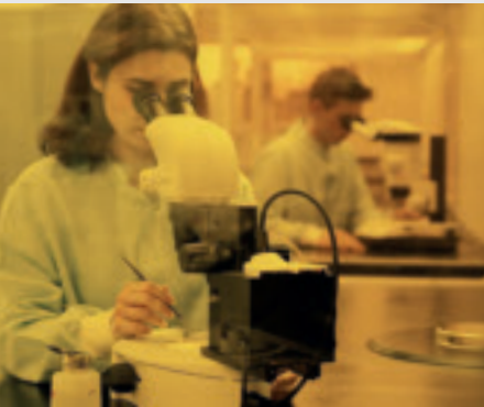
Leica S6 E with 38° viewing angle on a transmitted light stand
