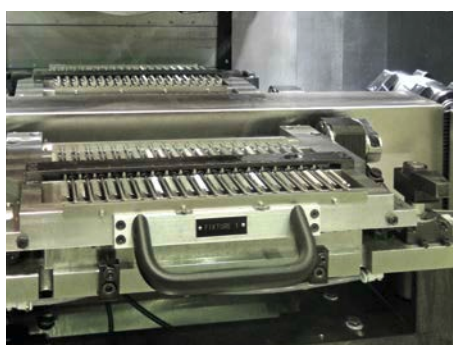
Index table with two clamping fixtures
